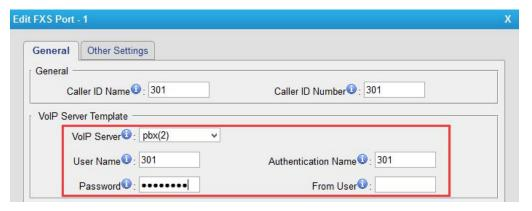
• **Template Register** – register to your VoIP server and apply the template to FXS ports.
